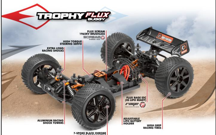
Formed from 4mm thick 6061 aluminum, the chassis of the Trophy Truggy FLUX features angled sides and a huge vertical rear brace for phenomenal stiffness front-to-rear. The twin batteries fit securely within an adjustable and padded battery box, held in place with two thick hook-and-loop strips so they won't move during jumps or crashes. The layout of the components within the chassis makes it easy to change batteries, and a breeze to do maintenance!
