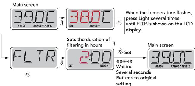
If Filter cycle 2 has been activated, Filter 12 is shown on the LCD display.
