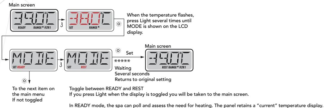
REST mode does not poll, and heating runs only during filter cycles. The panel does not always display the current temperature.
