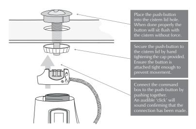
Once the 'command box' has been attached to the push button, lock the device by holding both sides of the coloured tab and pushing upwards until another 'click' sounds.
