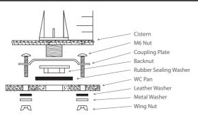
Fit siphon as described earlier but add coupling plate between the cistern and back nut. Ensure coupling plate is parallel to rear of cistern.
