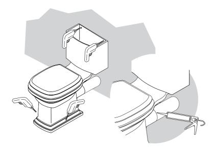
Operate the flush cycle a few times and continually check carefully for signs of leaks from the inlet valve or toilet outlet if no leaks are evident, your toilet installation is complete.
