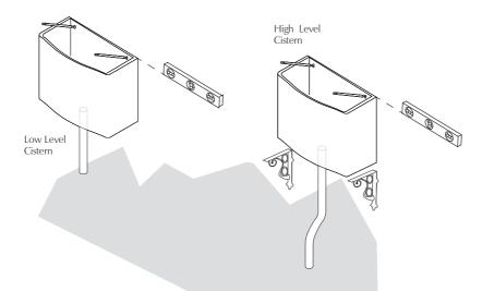
Once cistern is installed, fit the flush pipe to the bottom of the cistern but do not fully tighten until later in the installation.
