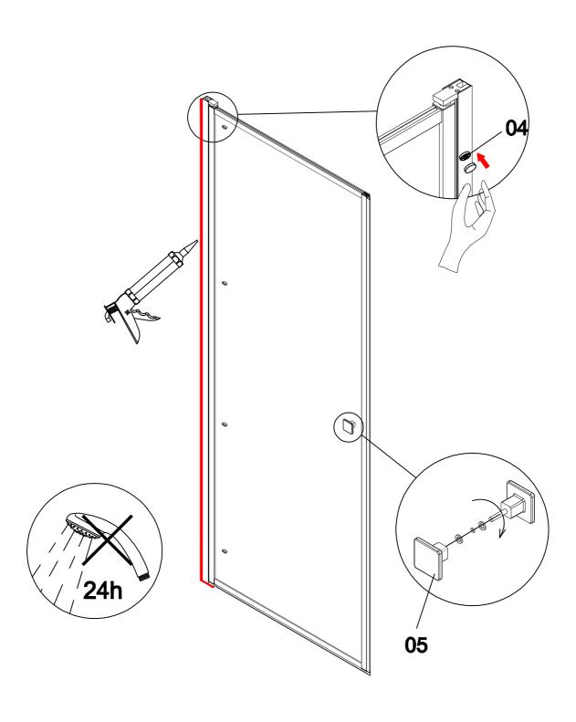
Before the final set up of this shower enclosure, check its watertightness. In case of leakage, retighten the screws and if necessary add silicone.
