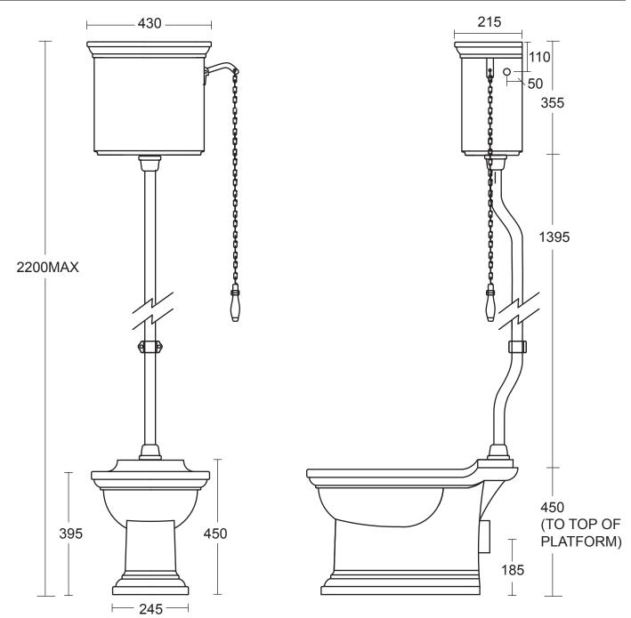
RADCLIFFE FLUSH PIPE = 1495mm (-100mm HIDDEN IN TANK+CLOSET) EXPOSED LENGHT = 1395mm
